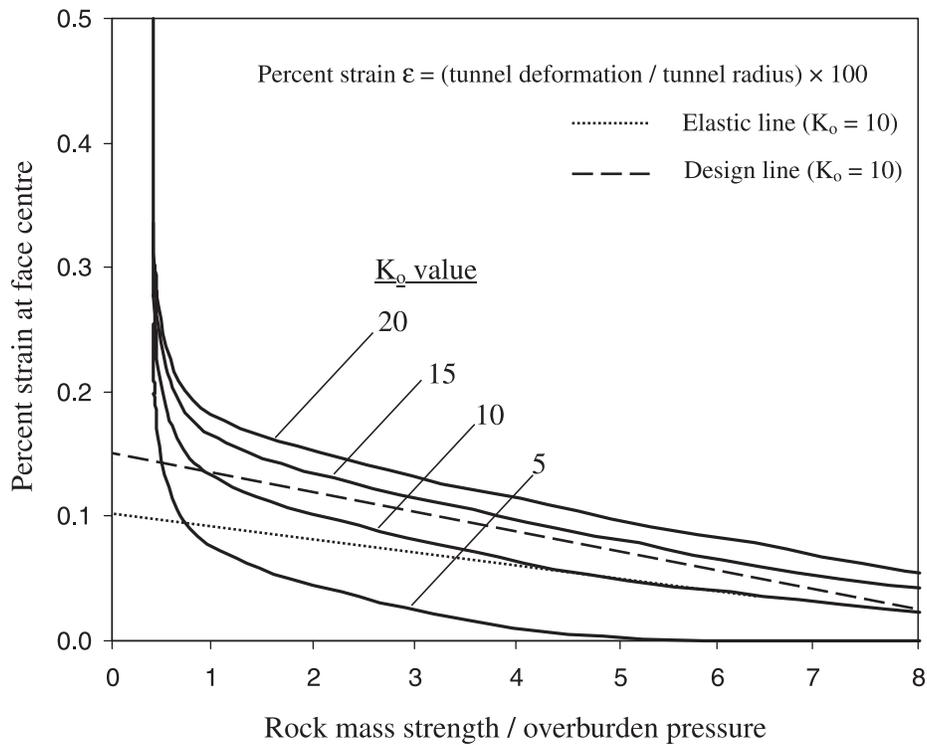
**Fig. 7.** The effect of rock mass strength reduction on the displacement at the tunnel springline.
