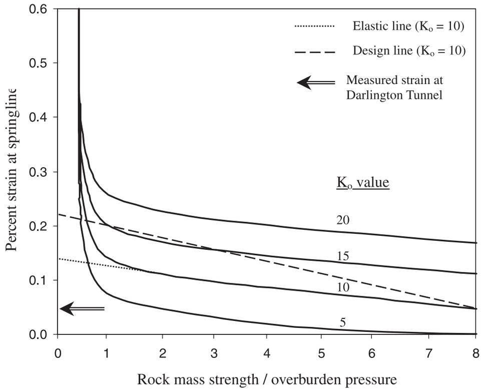
**Fig. 8.** The effect of rock mass strength reduction on the displacement at the tunnel crown.
