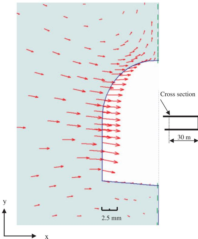
the tangential (horizontal) direction was calculated near the tunnel wall. This maximum compressive stress is well below the estimated compressive strength of the rock mass (80 MPa). The stresses in the radial direction were zero at the tunnel wall and increased to 3 MPa at a distance of 2 m and decreased to the overburden pressure (1 MPa) at a distance of 40 m from the tunnel wall.
