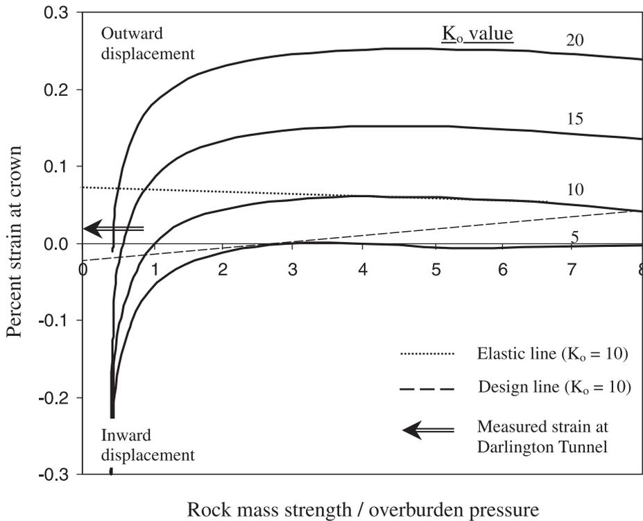
within tolerable limits. These limits will vary depending on the location of the point of interest within the tunnel circumference. The elastic and suggested design strains are summa-
