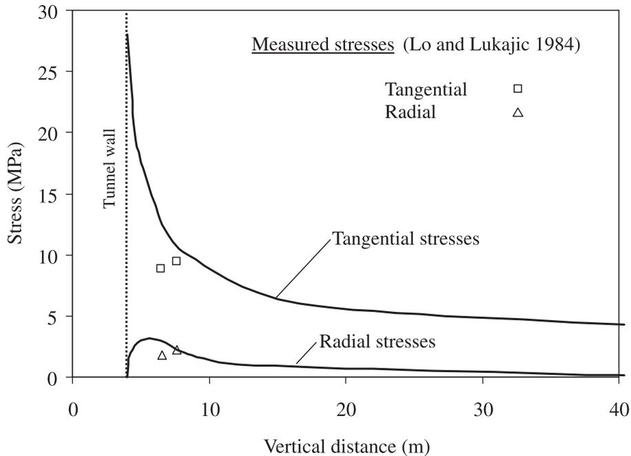
gested design lines were established for a  $K_0$  value of 10 as shown in Fig. 8. The strain was found to range between 0.07% and -0.04% at the tunnel crown. The measured strain at the crown of the Darlington tunnel was 0.02%, which fits between the elastic and the suggested maximum strain range, indicating that no stability problems are expected at the tunnel crown under the existing in situ stress conditions.
