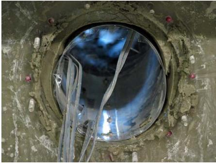
**Fig. 6.** Photograph of aluminum lining during gap closure process
