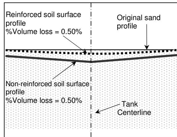
Figure 5: Schematic of surface profile following a subsurface volume loss
