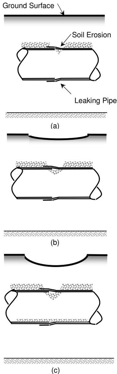
Figure 1: Soil response to subsurface erosion caused by a leaking pipe
