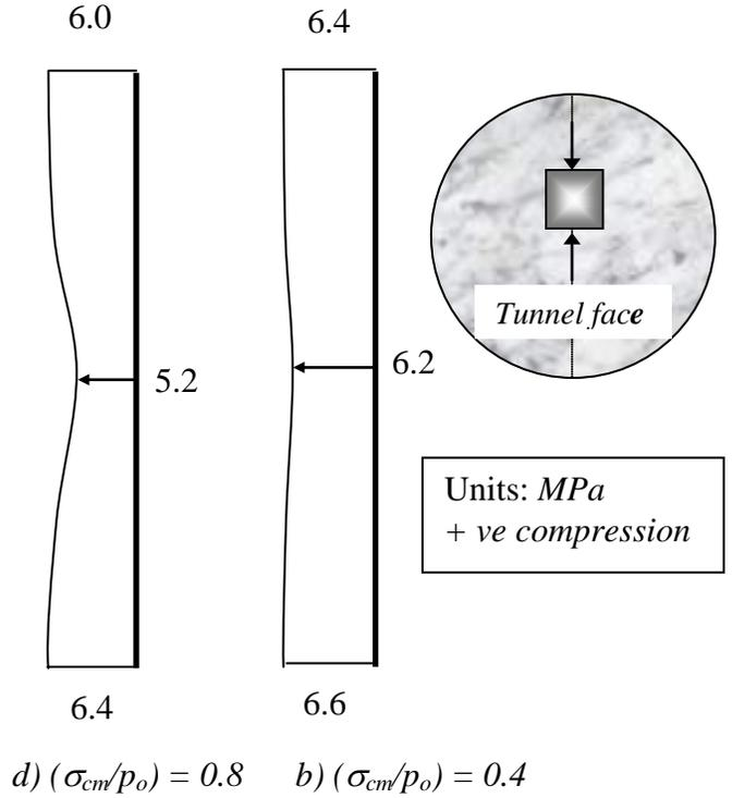
Figure 4. Distribution of tangential stresses at the tunnel face
