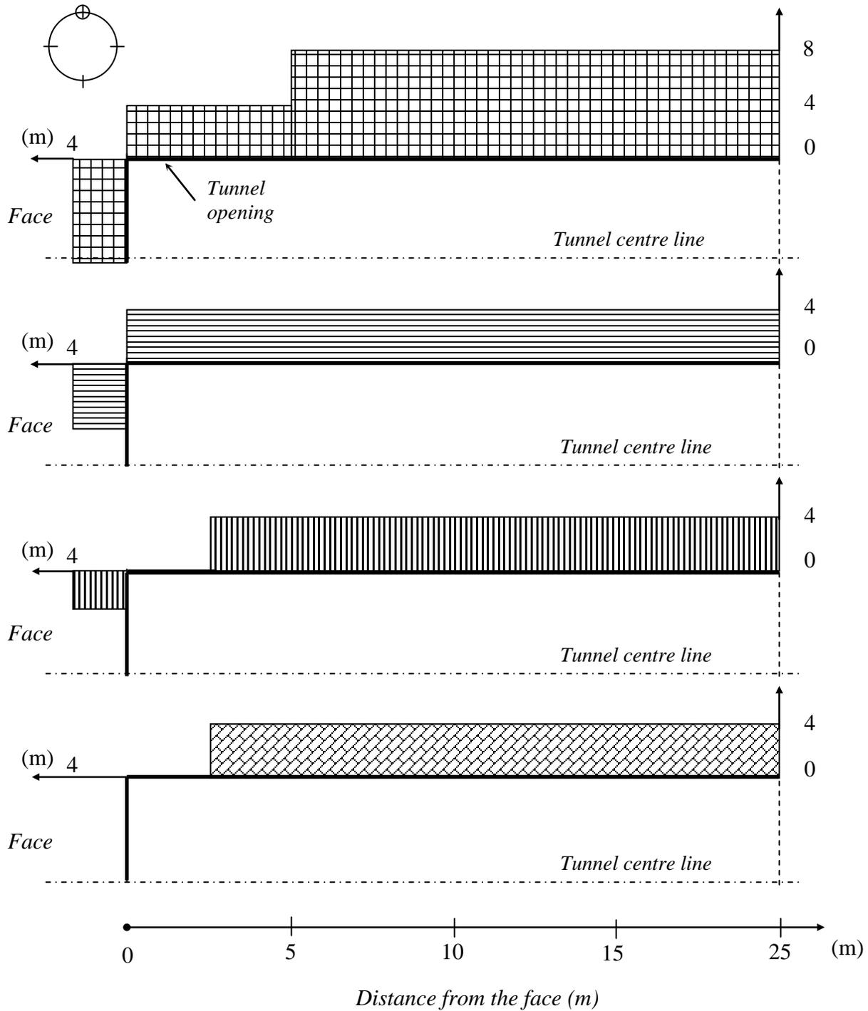
Figure 8(a) Approximate extent of plastic zone at the tunnel face and crown
