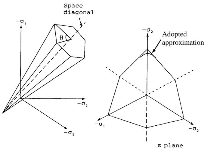
Figure 1. Mohr-Coulomb Failure Criterion in the principal stress space
