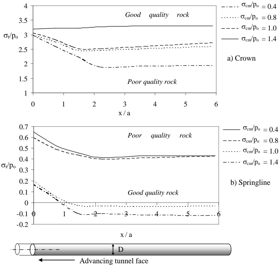
Figure 7. Variation of tangential stresses with distance from the tunnel face
