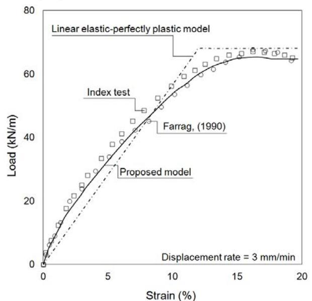
Figure 9. Unconfined (in-air) tensile test results on geogrid
