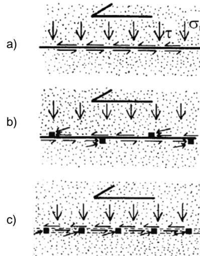
Figure 2. Interaction in direct sliding, a) sheet or strip reinforcement, b) ribbed strip reinforcement, and c) grid reinforcement, (after Milligan et al., 1987)
