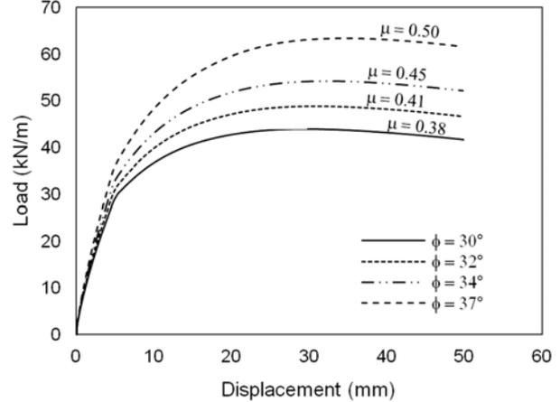
Figure 12. Effect of soil friction angle and interaction coefficient on geogrid pull-out load
