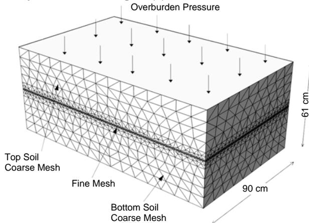
Figure 7. A complete finite-element mesh
