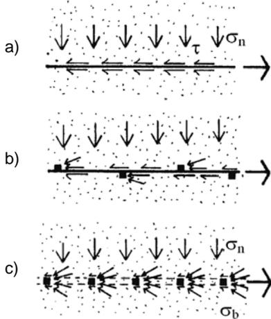
Figure 3. Interaction in bond resistance, a) sheet or strip reinforcement, b) ribbed strip reinforcement, and (c) grid reinforcement, (after Milligan et al., 1987)
