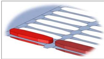
Figure 8. Soil-geogrid interlocking
