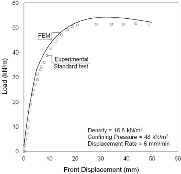
Figure 10. Pull-out response of the geogrid
