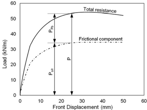
Figure 11. Components of the pull-out resistance
