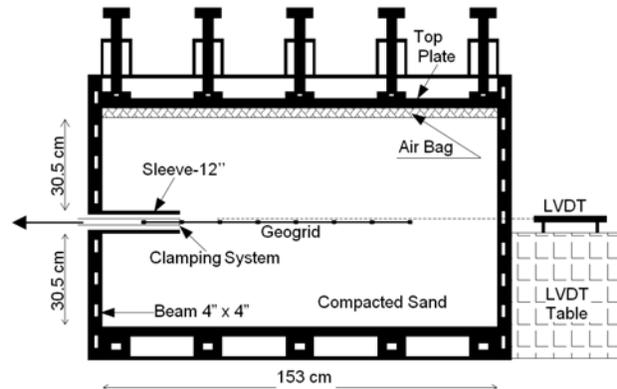
Figure 4. The pull-out box (adapted from Farrag, 1990)
