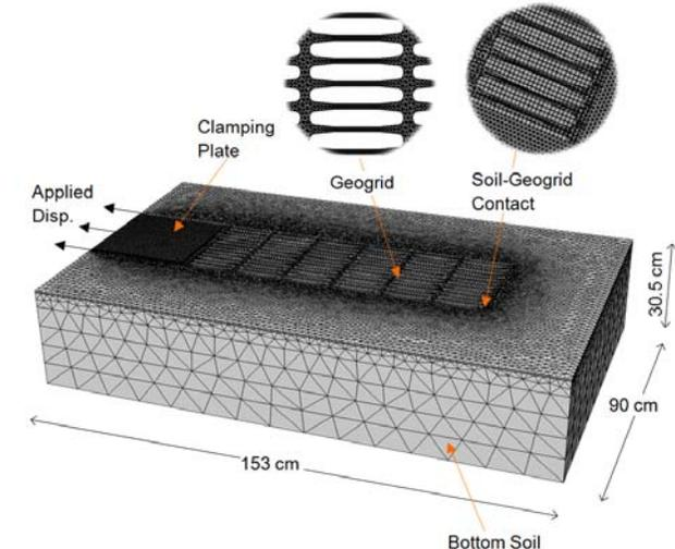
Figure 6. Finite-element mesh for the lower half of the box
