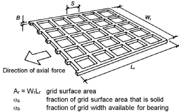
Figure 1. Definition of reinforcement dimensions (After Jewell et al. 1984)
