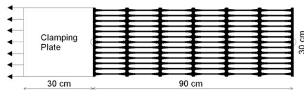
Figure 5. Standard geogrid specimen
