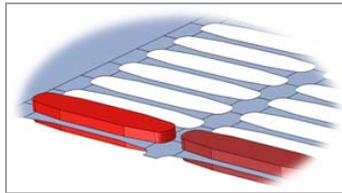
Figure 8. Soil-geogrid interlocking
