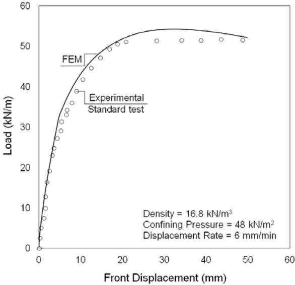
Figure 10. Pull-out response of the geogrid
