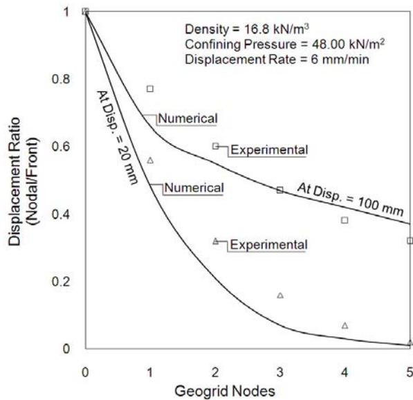
Figure 8. Distribution of displacement along the geogrid
