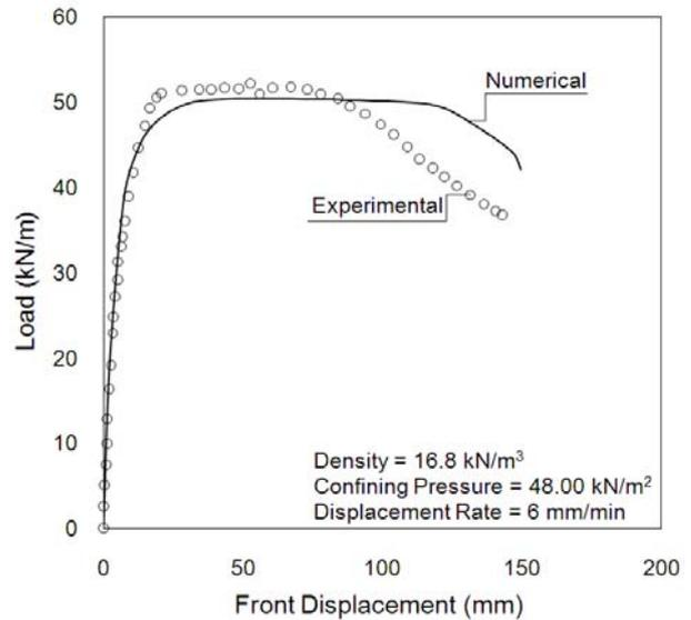
Figure 6. Pull-out test results on geogrid
