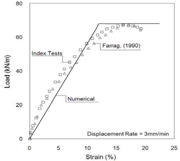
Figure 5. Unconfined (in-air) extension test results on geogrid
