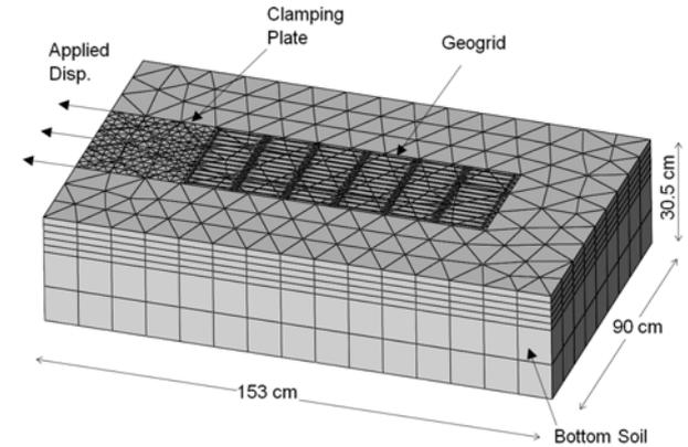
Figure 3. Model geometry showing the lower half of the box
