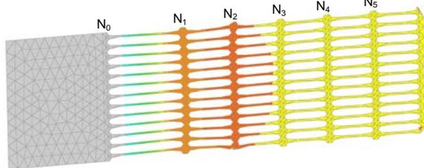
Figure 9. Deformation of geogrid during pull-out loading
