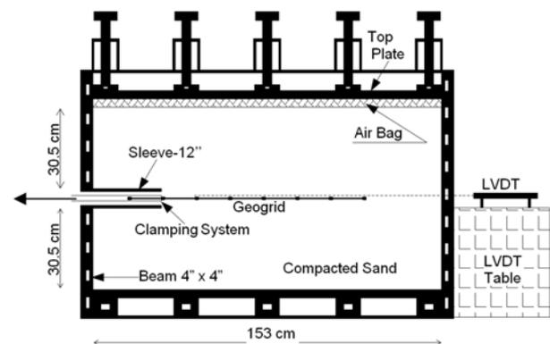
Figure 1. The pull-out box (Adapted from Farrag, 1990)
