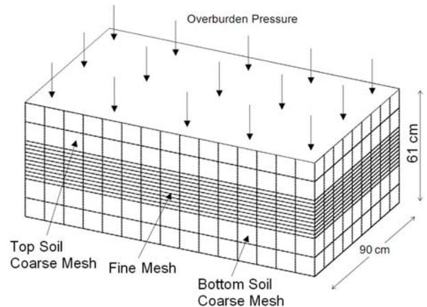
Figure 4. Finite-element mesh used in the 3D analysis
