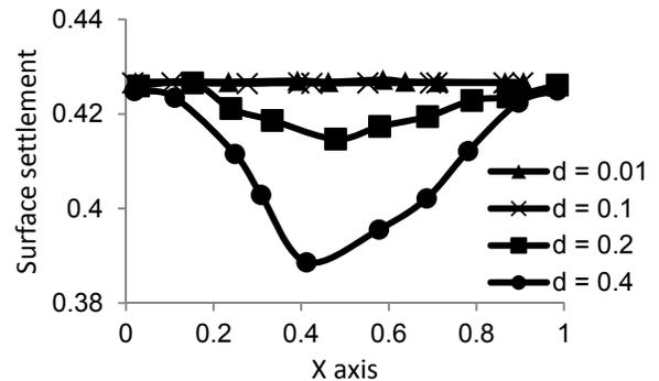
Figure 6 Effect of trapdoor displacement on surface settlement
