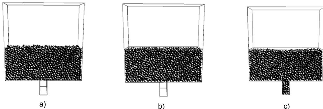
Figure 3 Snapshots of the three stages of simulation: a) initial packing; b) Top wall activated; c) Trapdoor activated
