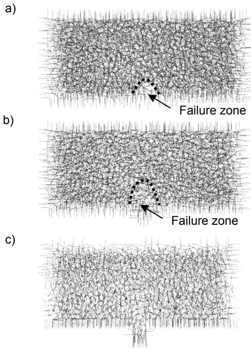
Figure 4 Force network for the different values of trapdoor movement: a) 0.01 m, b) 0.05 m and c) 0.4 m
